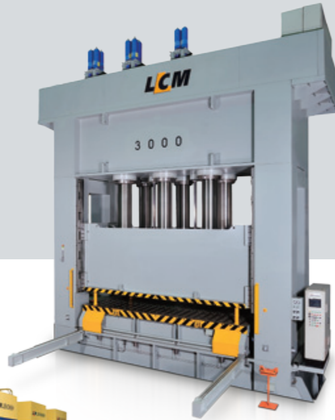
Tonnage: 3,000 ton Bolster Area: 6,000 x 2,500 mm
