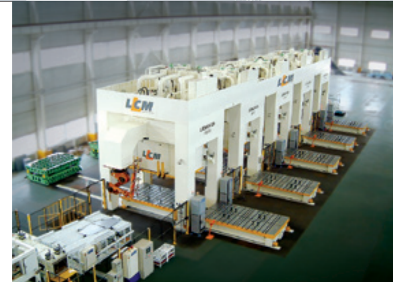
Fully Automated High Speed Hydraulic Tandem Line With Processing Equipment, Washing Unit, Centralizing System and Robots Tonnage: 800 ~ 1,600 ton Bolster Area: 4,600 x 2,500 mm
