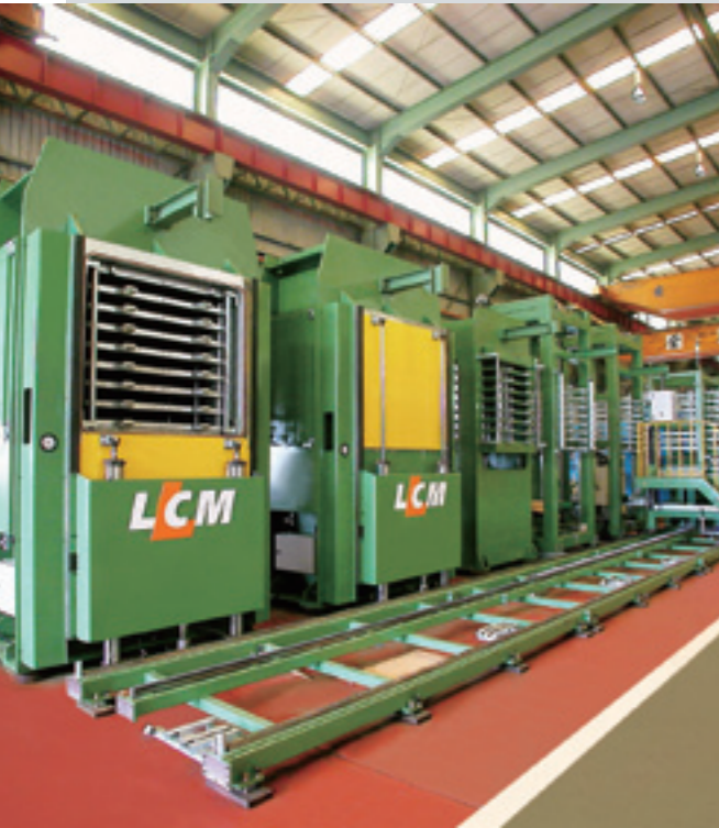
Tonnage: 720 ton , 8 Openings Platen Area: 1,220 x 1,370 mm
