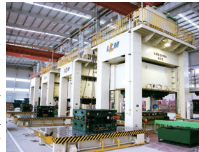
Manual Loading Hydraulic Tandem Line Tonnage: 600, 800 and 1,200 tons
