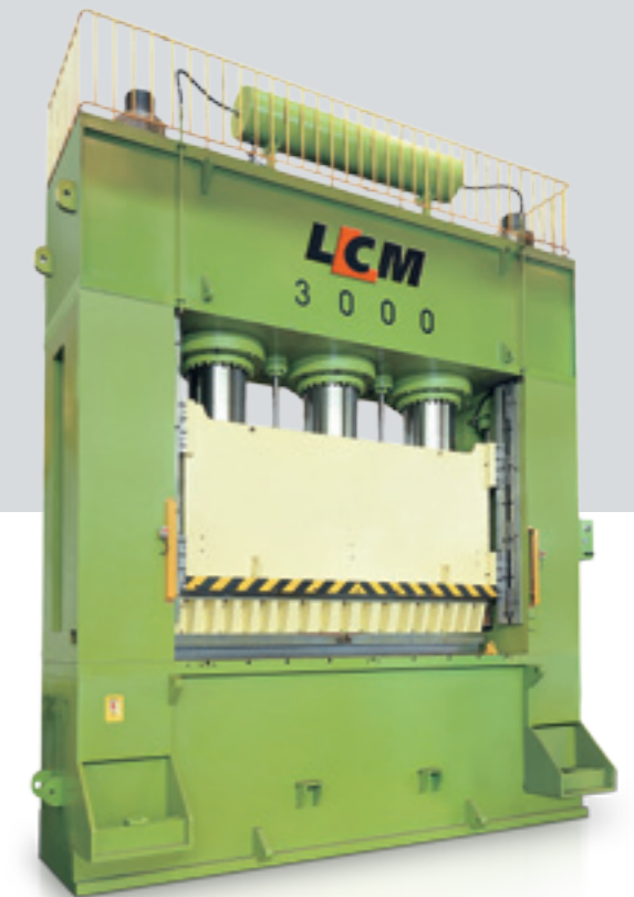
Tonnage: 3,000 ton Bolster Area: 4,600 x 1,800 mm
