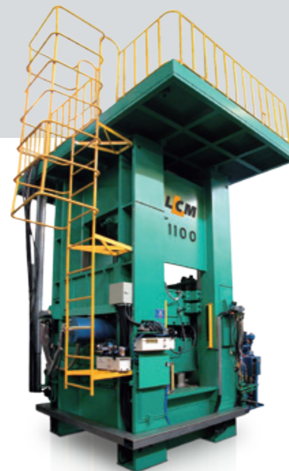
Tonnage: 1,100 ton Bolster Area: 1,800 x 1,200 mm
