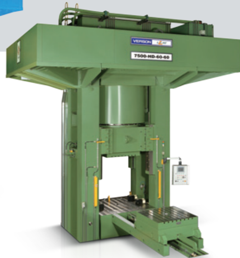
Tonnage: 7,500 ton Bolster Area: 1,524 x 1,524 mm
