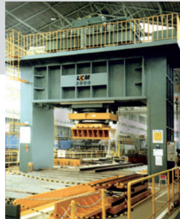
Traveling Ram Hydraulic Shipyard Press Tonnage: 3,000 ton Bolster Area: 5,600 x 2,500 mm
