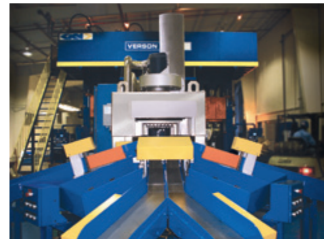
Hydraulic Warm Forging Press Tonnage: 400 ton Bolster Area: 805 x 750 mm
