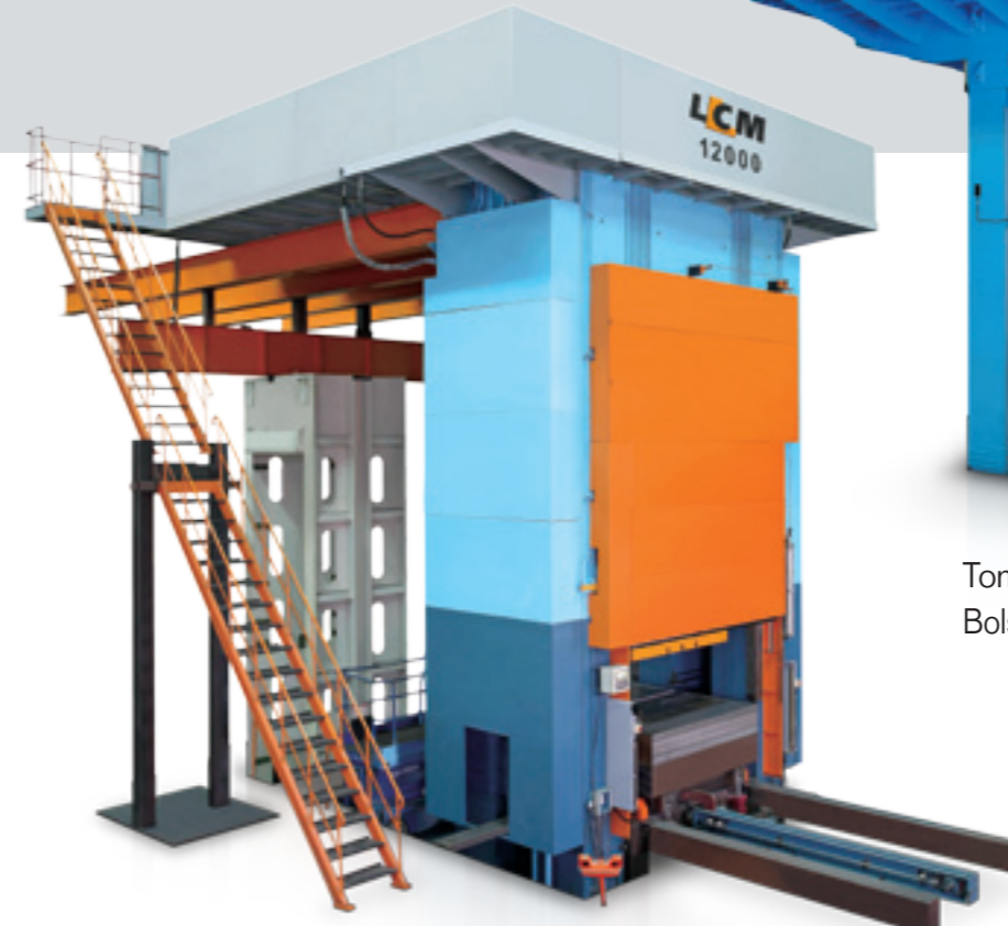
Tonnage: 12,000 ton Bolster Area: 2,700 x 2,500 mm
