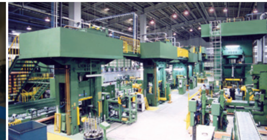
Fully Automated Shell Forging Production Line Tonnage: 125 ~ 3,000 ton Bolster Area: 810 x 950 mm / 810 x 1,150 mm / 915 x 1,095 mm / 1,375 x 1,675 mm / 1,525 x 1,880 mm
