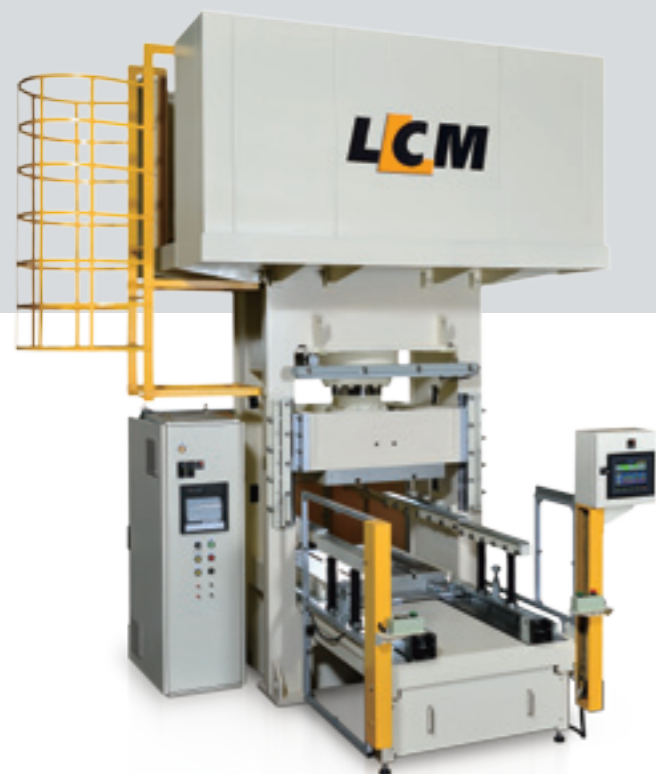
Tonnage: 200 ton Platen Area: 900 x 700 mm
