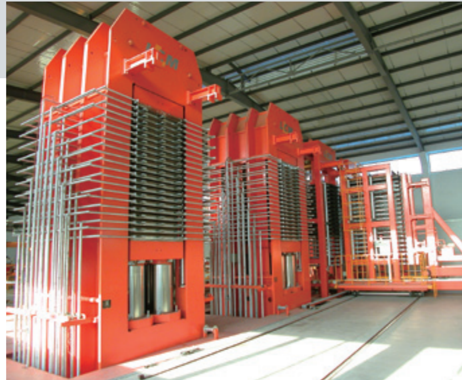
Tonnage: 3,500 ton , 20 Openings Platen Area: 1,370 x 2,300 mm
