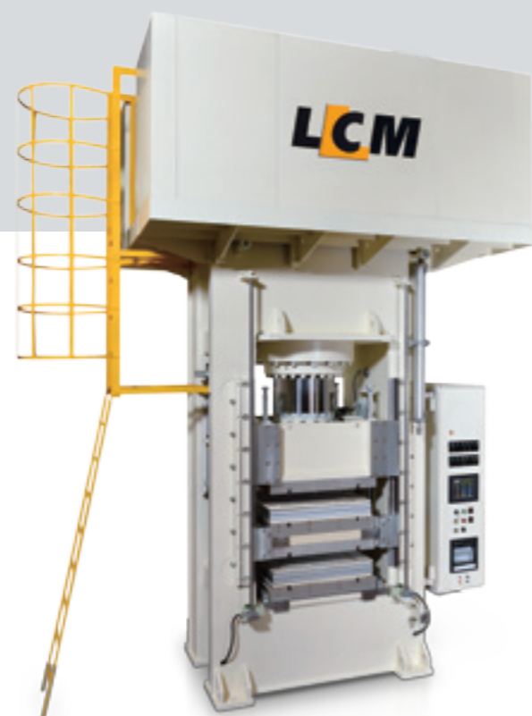
Tonnage: 500 ton Platen Area: 900 x 900 mm
