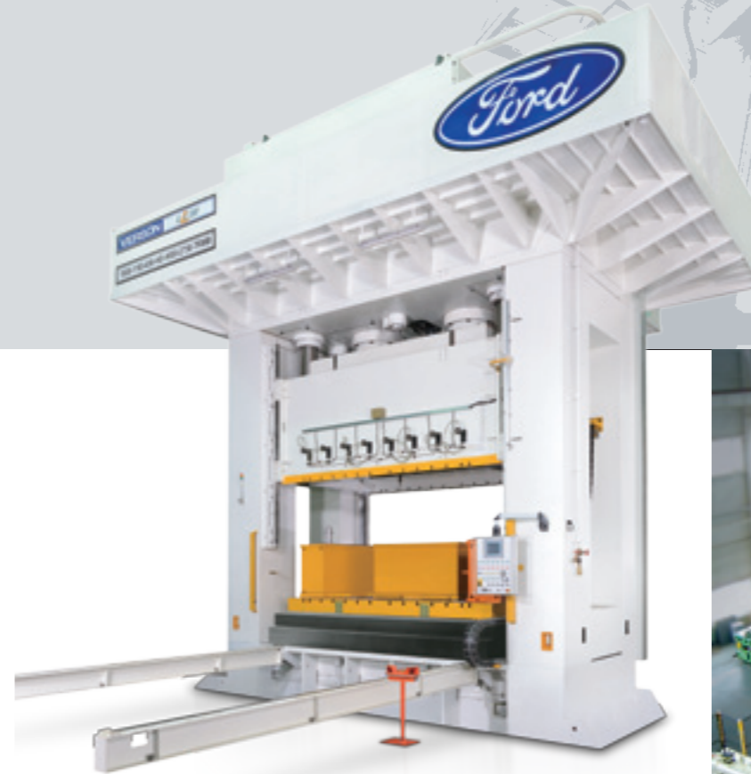
Tonnage: 3,000 ton Bolster Area: 6,000 x 2,500 mm
